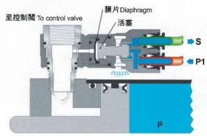
P': 壓力排出/Exhaust pressure P:系統壓力/System pressure
